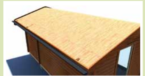
Second T and G ceiling to sandwich insulation
