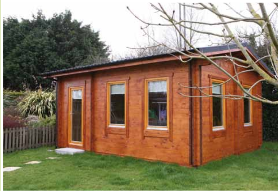
Twin log walls are made up of 2 x 45mm solid logs with 50mm rock wool insulation sandwiched in between.
